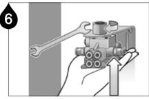
Connect the divider block to the adaptor. washer, and mounting bracket and turn the adaptor (A002) clockwise to tighten.
