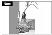
Prefill the divider block with the same or compatible grease using a grease gun and a 3/8" grease nipple.
