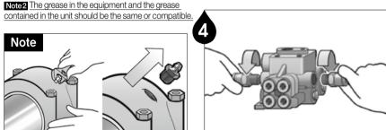
Screw in the push-in fitting connectors to each port of the divider block.
