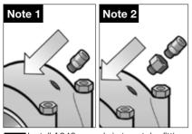
Note1 Install A240, a push-in type tube fitting, directly onto the lube point.
