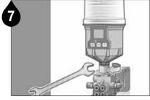
Install the lubricator onto the mounting bracket using a 17mm wrench.
