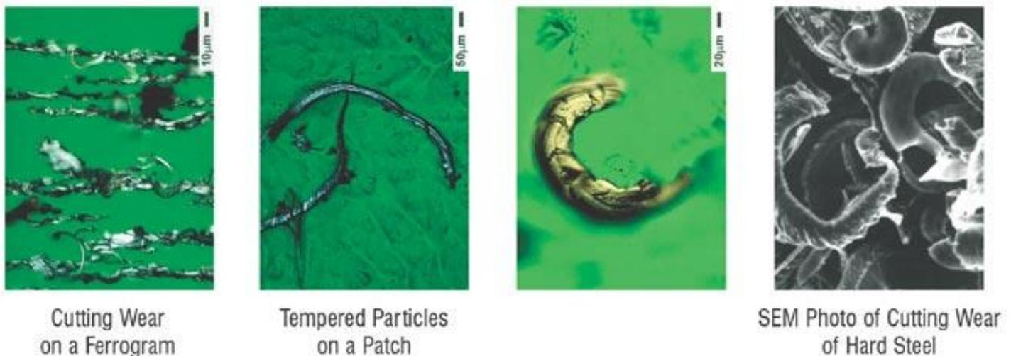
Figure 7. These Ferrographic Images are Typical of the Shape of Wear Particles Produced by Three-body Abrasive Wear.
